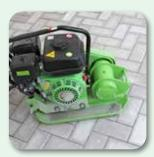
Compact the material by using a wacker plate
